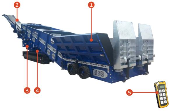
30yds<sup>3</sup> hopper capacity with dual access, hydraulic flared sides and truck ramps.
